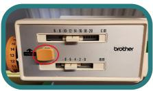
You can test that the sheet is advancing by the correct amount by carrying out a simple test. You know from your swatch how many centimetres you get for 60 rows of knitting. Mark two lines on your charting sheet that many centimetres apart, line up the lower line with your charter and 'knit' 60 rows without any yarn or needles selected. You should end up at the upper of the two lines. If you prefer, you can calculate the number of rows in 10cm by doing a little bit of maths (or using a green
